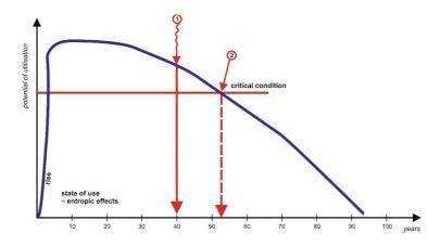
Fig 2. Seneca cliff in reference to a building structure; two moments of the structure withdrawal from use are marked; exceeding the critical condition: 1 – as a result of entropic effects; 2 – as a result of entropic effects and impact of an external factor
